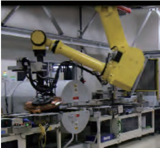
Automated inspection system utilizing an arm robot
